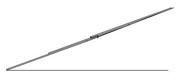
4. Hammer one edge of slate with slate hammer, and slide repair piece of slate into place just above the hook. Slide the slate down until the notch made with hammer rests in the hook
