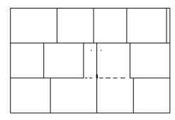
2. Line up the hook end of the slate hook with bottom edge of slate on both sides of missing piece
