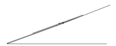
3. Hammer spike end of hook in-between two pieces below to roof deck
